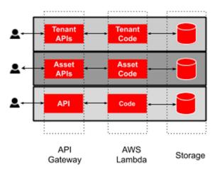
Each API group runs inside a dedicated virtual network and uses AWS's Identity and Authorization Management system to control access to resources. The IAM permission system follows the principle of least privilege, ensuring every resource has permissions to access only exactly what it needs based on the processing needs.
